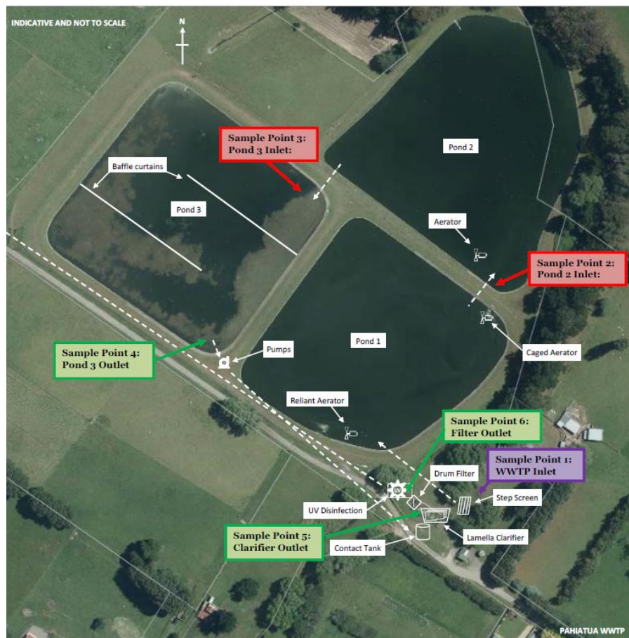
Figure 1 - Layout of Treatment Plant Upgrades
